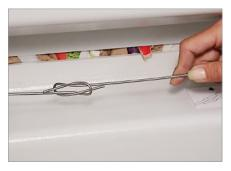
**Strapping** Manual bale strapping with Quick-link wire.
